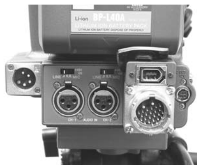
On the Sony DVCAM, you set the audio inputs for either mic or line level, depending on your source signal.
