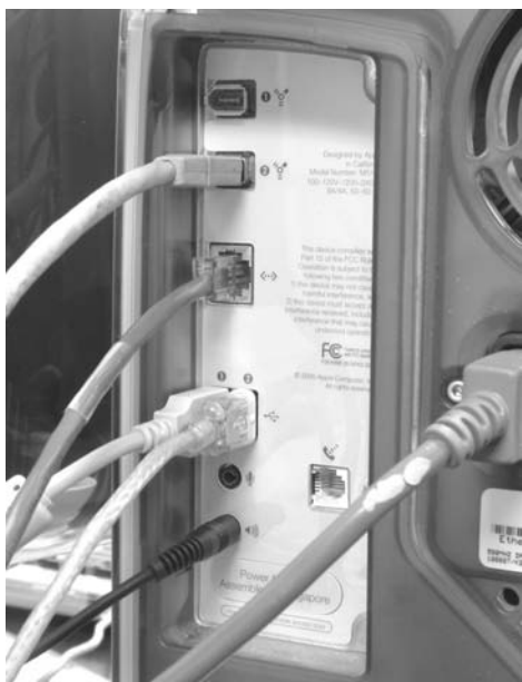
To get a digital signal into your computer, there must be an appropriate and functioning input. The input might be there, but it may be attached to nothing inside the computer.
