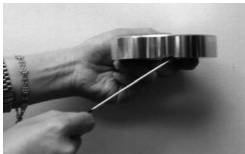
The tiny video head is mounted at the base of the head drum.
