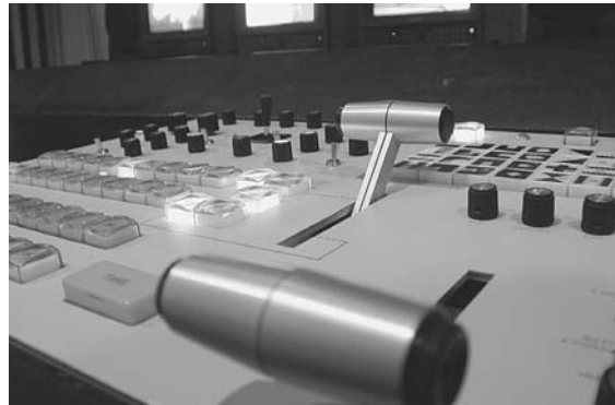
These controls decide the signal which goes to broadcast or to tape. (Photo from Northern Melbourne Institute of TAFE)
