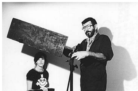
A C-stand can hold a cutter or black flag to shield an area on set from direct light. Vicki Lucan and Ken Crouch, Australian Film Television and Radio School.
