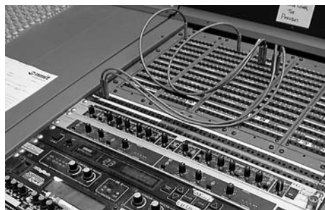
Routing audio through a patch bay, Northern Melbourne Institute of TAFE, Collingwood, Vic, Australia.
