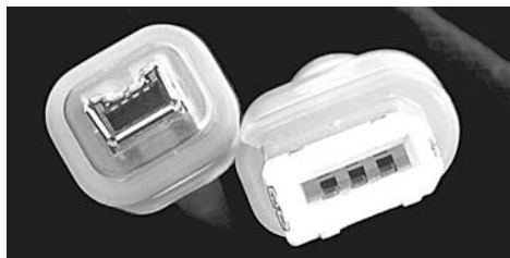
The FireWire connector is used when sending digital video into and out of a computer. It's also used to attach other equipment to a computer.
