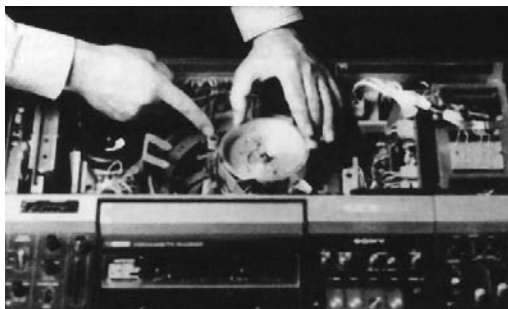
The video head drum spins in the opposite direction to the tape travel.
