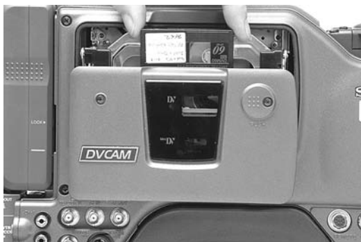
Sony DVCAM can take both small and large tapes.
