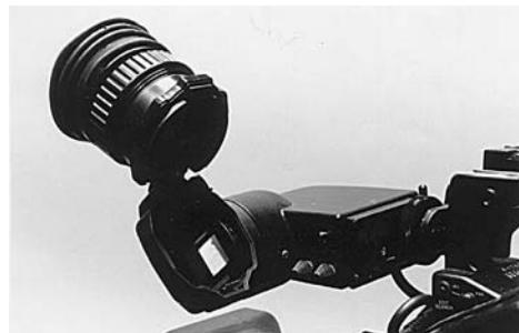
Diopter open—an option for tripod operation.
