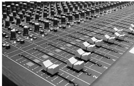
Each fader knob controls the volume level of the signal attached to one sound input.
