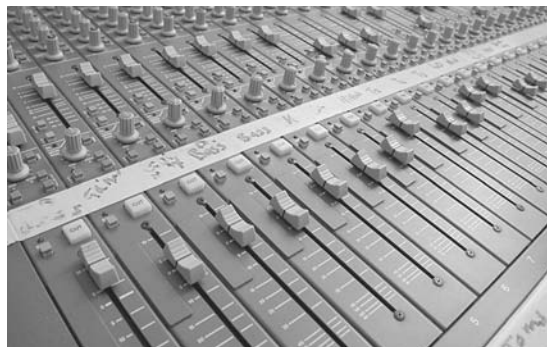
Masking tape is commonly used to label which signal is going to which fader. Tape can also be used to mark the right level for each fader. (Photo from Northern Melbourne Institute of TAFE)
