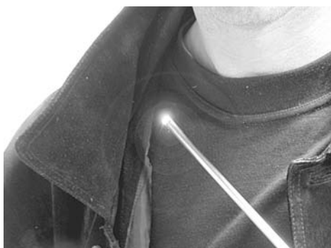
The endoscope lens is very tiny and comes on a long flexible lead with a light mounted next to it.
