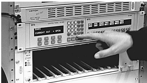
The routing switcher lets you select a signal and send it to whatever equipment you choose.
