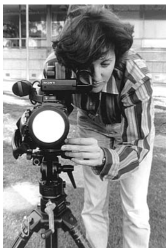
Bronwyn Gell does a white balance on the white lens cap, Hamilton Secondary College, Mitchell Park, SA, Australia.
