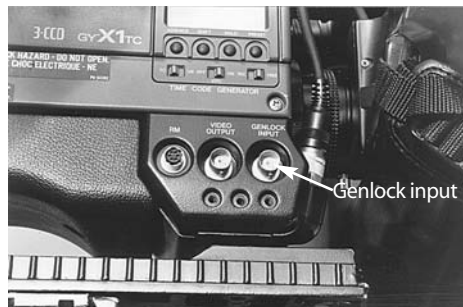
The sync signal from the studio sync generator, or some other timing device, is fed to the camera through the genlock input.
