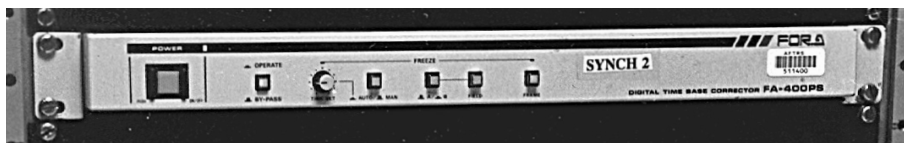
A frame store does the same job as a TBC, but it can also do additional special effects.
