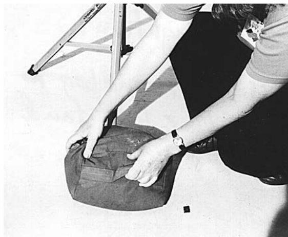
You can secure lightstands with sandbags.
