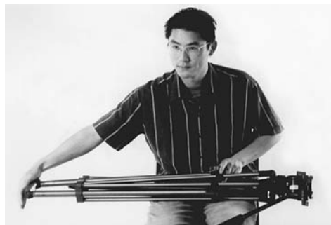
Lengthen the tripod legs evenly before you open them. Gunther Hang, AFTRS.
