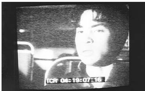
Timecode burn-in can be put anywhere on the picture, but it's usually put on the bottom.
