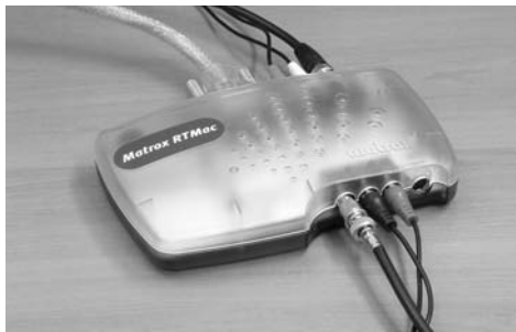
This Matrox handles both analog and digital signals in and out of the computer.
