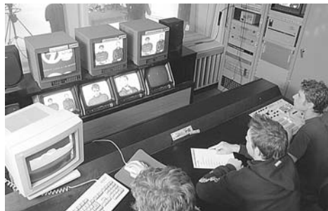
In this control room the crew can use either the TV monitors or the glass window to check what's happening on the studio floor. Northern Melbourne Institute of TAFE, Collingwood, Vic, Australia.
