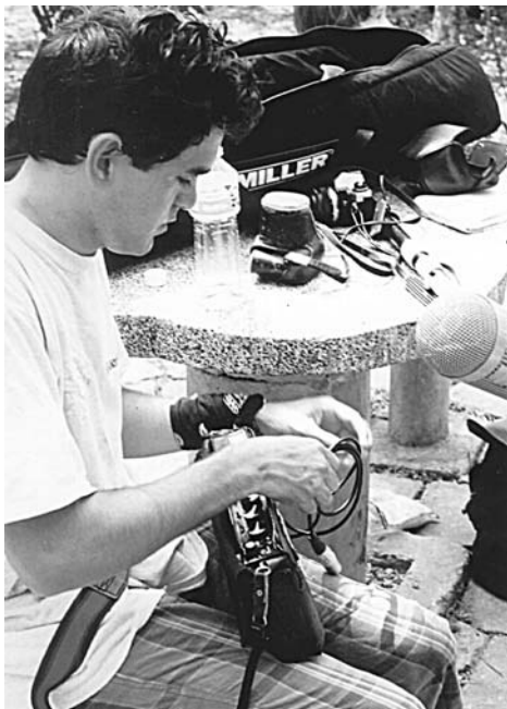
With a mixer you can input more than two mics at a time. Jason Troutman on location in Xishuangbanna, Yunnan, China, for Dai Women Speak . (Photo by Michelle Blakeney)
