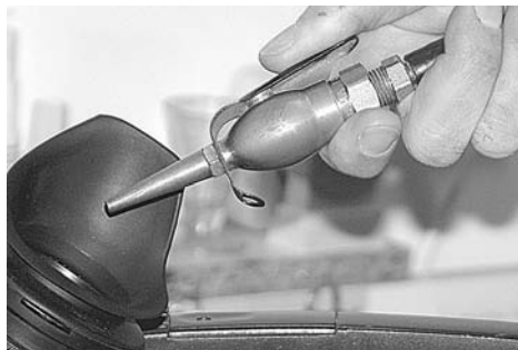
Pressurised air can clean fine particles from the lens without scratching it.
