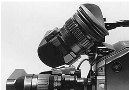
Diopter closed for handheld operation.
