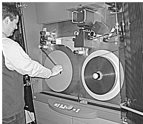
Craig Dingwell threads film onto a telecine machine. (Courtesy of ScreenSound Australia)
