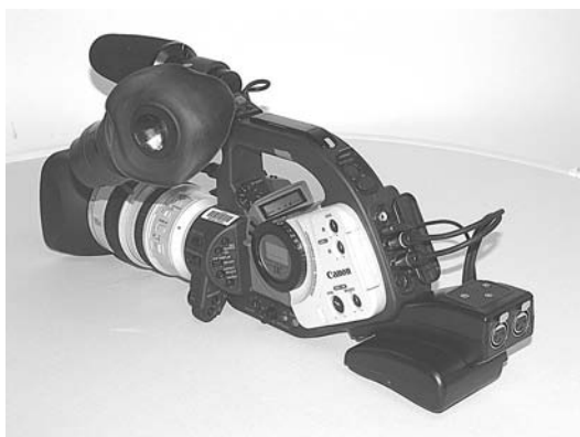
The Canon DV camera has an adaptor which allows two XLR audio inputs at the back.
