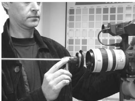
The endoscope lens attaches to the front of the camera lens, shown here by Julian Ellis, cinematographer.
