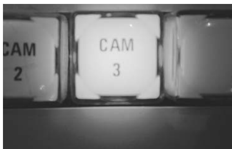
The vision mixer lets you select any source which is connected to it, by pressing the corresponding button. (Photo from Northern Melbourne Institute of TAFE)
