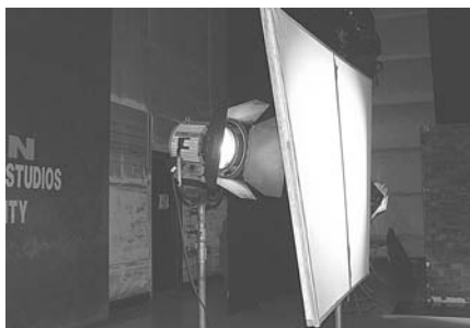
A light shining through a diffusion screen provides a soft light for the actor in front of the window frame.
